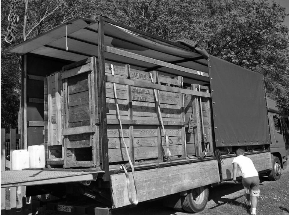
**Figure 2.** During transport, containers should be secured to the board of the vehicle to prevent displacement (Fot. Michał Krzysiak)
